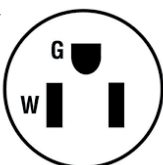
Plug Configuration NEMA 5-15P
